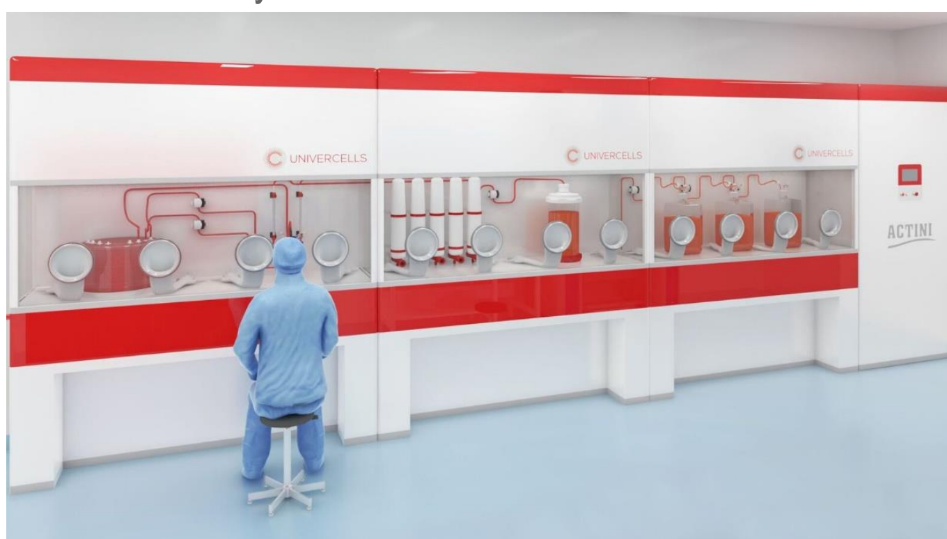
Figure 1: NevoLine single-use manufacturing platform, and its containment in BSL3 POD & POD-based facility
